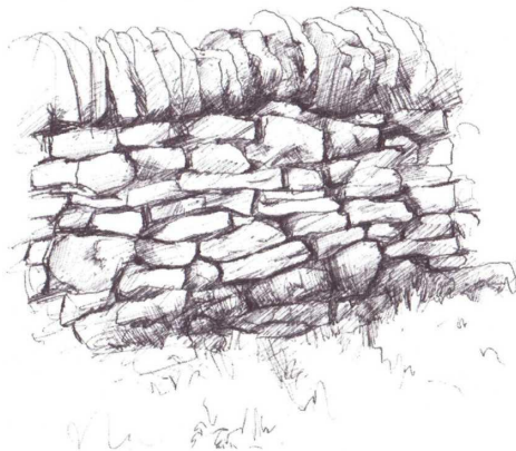
Typical section of dry stone walling.
